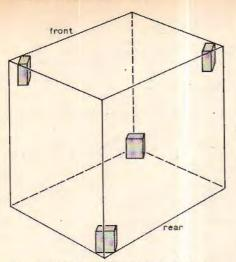
Fig. 3. Tetrahedral loudspeaker layout shown embedded in a cube.
